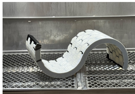
Before: FDM Part Before Support Removal
