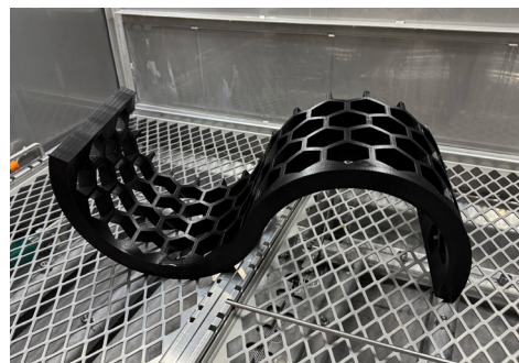
After: FDM Part After Support Removal in the BASE
