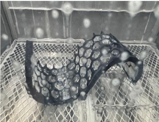
CIDEAS FDM Part Being Processed in the PostProcess BASE
