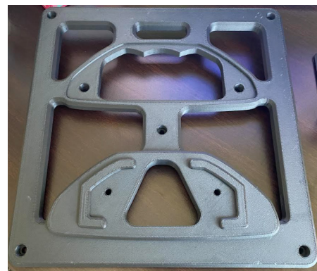
3D printed pallet used in J.W. Speaker's lighting production
